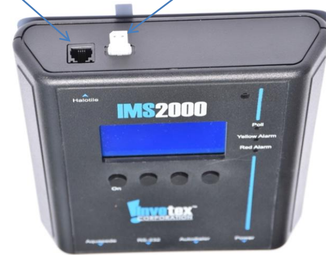
IMS 2000, Top End View, Halotile Connections
